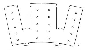
FIG. 71. Field core stamping of electrical steel for revolving field alternator (Westinghouse) showing bolt holes for assembling and securing sheets.
